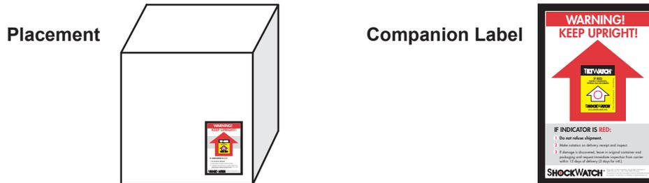
3. Press the TiltWatch XTR firmly in the center and around the edges to ensure strong adhesion to the container to which it is being applied.
