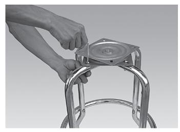
**Step 3:** Place swivel on top of legs and align holes. Top plate 45° angle to the other. Insert large bolts and screw on lock nuts securely. If swivel is tight place it on a carpeted floor, stand on it and twist, you should be able to turn it smoothly.
