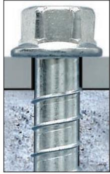
**Reinstallation of Titen HD® screw anchor in Original Drilled Hole**
