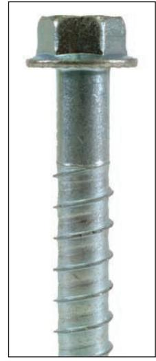
The Titen HD® screw anchor 3/4 x 6 and 3/4 x 7 (models THDT75600H and THD75700H) have a 1" section under the head that is unthreaded to allow installation into tilt-up wall braces.
