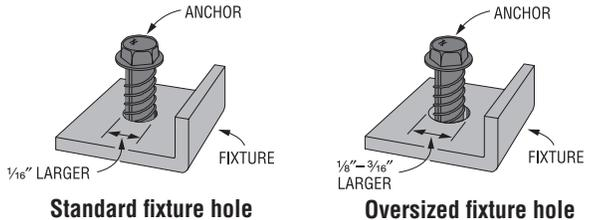
Use the following table to identify which diameter Titen HD® screw anchor to use based on the fixture hole type and diameter. In most cases where a smaller diameter Titen HD anchor is called out in comparison to the competitor's larger diameter anchor, the Titen HD anchor still generally provides allowable tension and shear load values comparable to or greater than those of the competitor's anchor.
