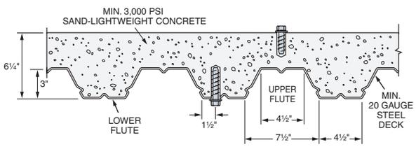
**Figure A – Titen HD® screw anchor installed in the top and bottom of a structural sand-lightweight-concrete and metal-deck assembly**
