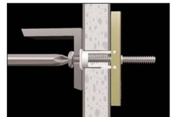
Place item over flange. Insert bolt and tighten until snug against item, then stop. Use machine screw or bolt to match thread in metal channel.
