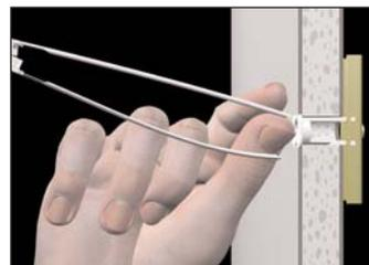
Place thumb between straps at wall. Push thumb side to side, snapping off straps level with flange of cap.
