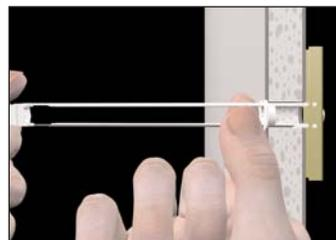
Hold ends of straps together between thumb & forefinger and pull toward you until channel rests behind wall. Ratchet cap along straps with other hand until flange of cap is flush with wall.
