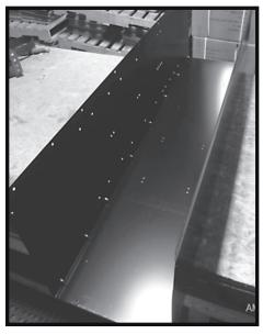
**Step 2:** Line up the holes in the center of the Side Panel with the center of the Back Panel. Attach sides using the Nuts and Bolts provided.
