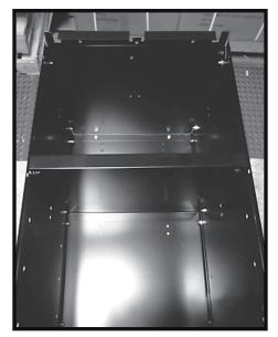
**Step 4:** Attach Shelf using the Nuts and Bolts. Tighten securely.
