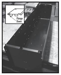
**Step 3:** Attach Top and Bottom Panels to the Side Panels and Back Panel with flange facing downward as shown. Secure with nuts and bolts.
