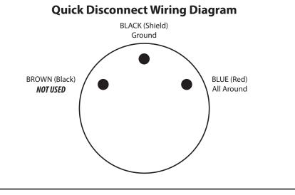
There are three wires in the supplied mating yellow/black cable, however you will only use <u>two</u> wires for the All Around (RED) Light (#LXAA-RED). The proper connection for these wires is shown in the following diagram:
