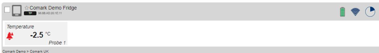
Clicking the measurement channel shows detailed alarm information and gives options to acknowledge or Reset the alarm.
